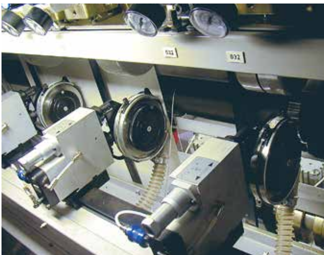
Suction casing mounted on slitter knife in printing press
