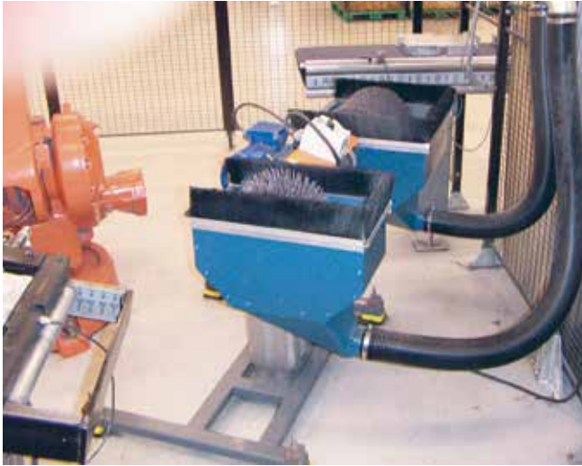
Robot deburring for telecom parts
